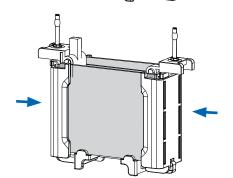
7. Place buffer tank on a level surface with the fill level indications facing forward. Place the primary electrode core inside the buffer tank, positioned between the lid alignment tabs. Ensure the anode and cathode leads are on the correct sides (red on right side). The alignment tabs on the tank will guide correct lid positioning. If buffer core is installed incorrectly, inner lid tab will prevent lid sealing.
