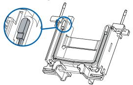
3. Open electrode core clamps by sliding clamps outward. Place the opened electrode core on a flat surface.
